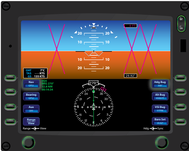
Figure 2-7. A PFD indicating a failed air data computer.
