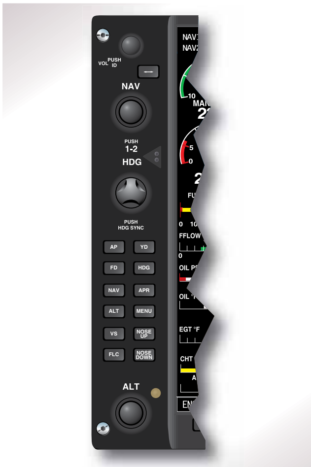
Figure 4-3. An integrated avionics system with an autopilot.
