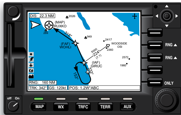
Figure 5-24. An instrument approach procedure shown on an MFD.
