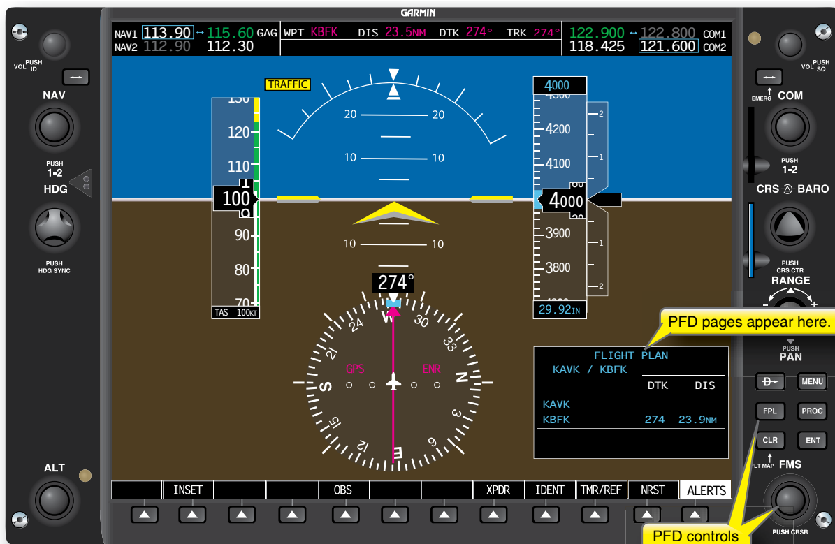
Figure 3-6. An integrated avionics system.
